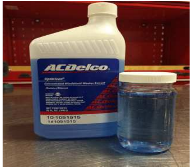
Diesel Exhaust Fluid (DEF) mixed with Windshield Washer Fluid.
