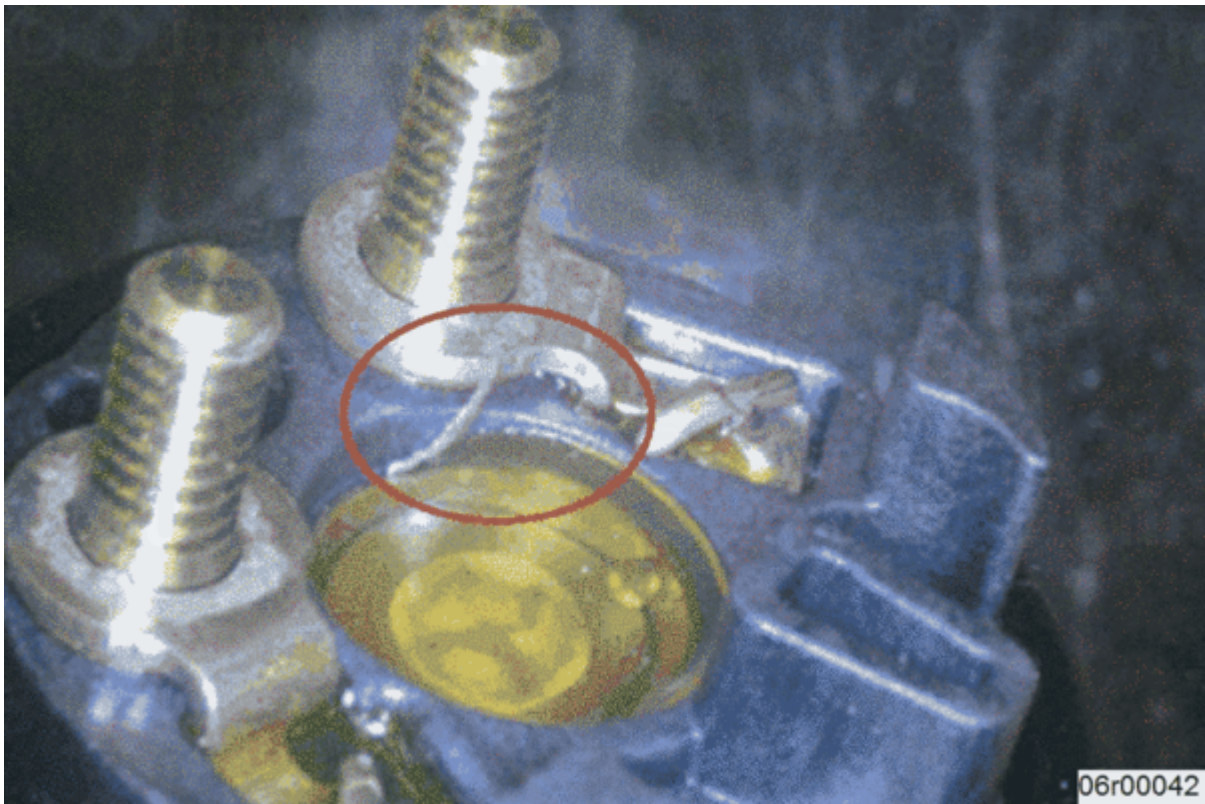
Figure 1, Injector Stator Contaminated With Metal Debris.
