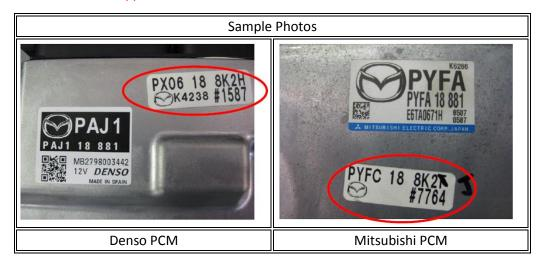
2. Launch MDARS by selecting "Start". If a connection is not possible after two tries due to IG OFF, MDARS starts the manual entry mode (forced ignition ON). Enter the VIN and the PCM software number.
