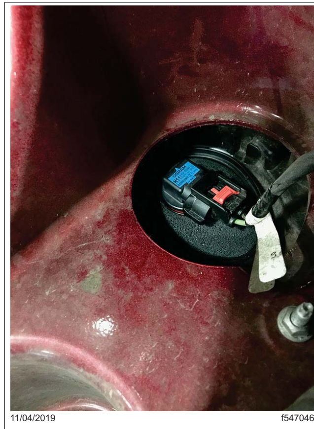
Fig. 8, Bulb Installed with Foam Grommet
