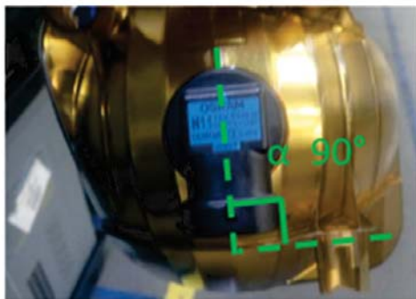
Fig. 11, View Through Headlamp Lens to Verify Bulbs are Fully Seated
