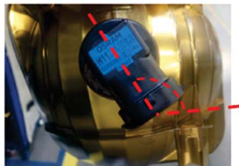
Fig. 11, View Through Headlamp Lens to Verify Bulbs are Fully Seated
