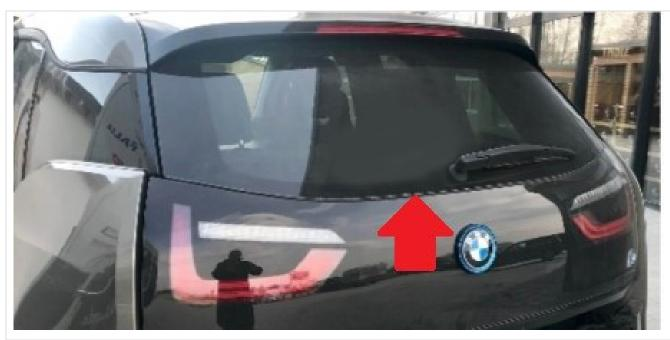
The rear window may be improperly bonded in the area shown above (red arrow), which could allow water to enter the luggage compartment.
