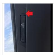
1. Inspect the status LED on the door release switch as shown to the left.
