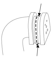
Alternator Cover Grommet Sealant Path
