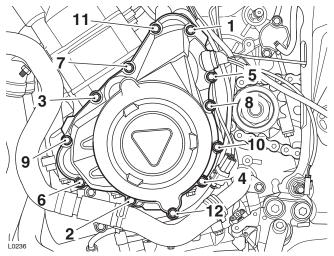
Alternator Cover Fixings Tightening Sequence
