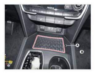
Using a flat head screwdriver or trim removal tool, remove the console upper cover (C).
