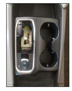
**7.** Re-assemble the upper console assembly so the assembly points align with the floor console.
