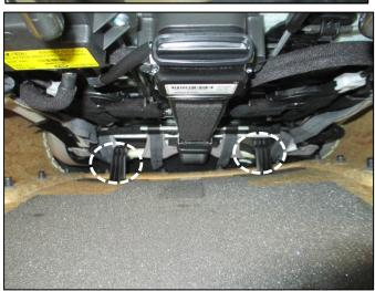
3. Lay the seat backboard on a clean workbench and inspect base clips (C).
