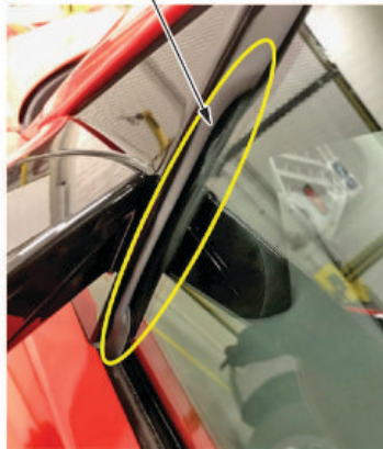
OUTER DOOR SEAL PINCHED
