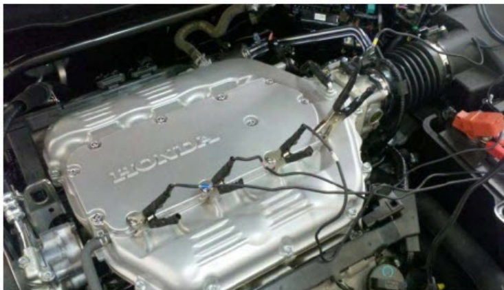
ChassisEar pickups mounted to Intake Manifold
