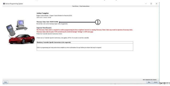
**Note:** To avoid warranty transaction rejections, you **MUST** record the warranty claim code provided on the SPS Warranty Claim Code (WCC) screen on the job card. Refer to callout 1 for the location of the WCC on the SPS screen.
