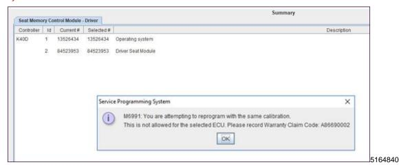
**Note**: If the Same Calibration/Software Warning is noted on the SPS Summary screen, record the warranty claim code (WCC) and select OK and follow screen instructions. If programming is completed, the WCC is located in the Service Programming System dialogue box of the SPS Summary screen. No further action is required. Refer to the Warranty section of the bulletin.
