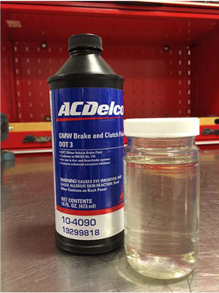
Diesel Exhaust Fluid (DEF) mixed with Brake Fluid.
