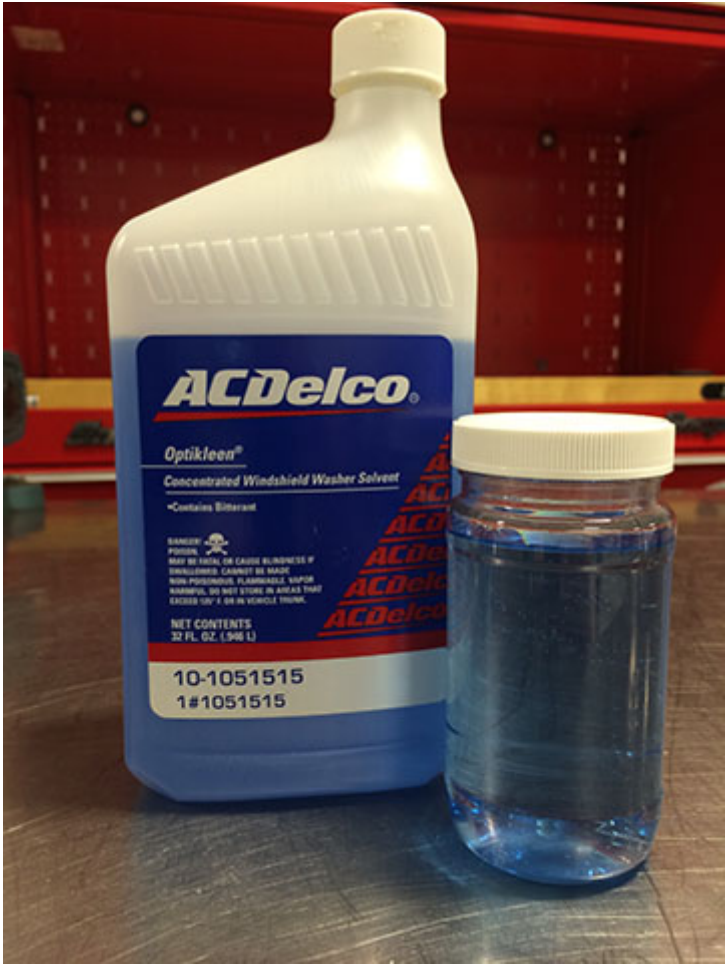
Diesel Exhaust Fluid (DEF) mixed with Windshield Washer Fluid.
