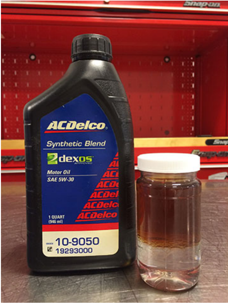
Diesel Exhaust Fluid (DEF) mixed with Engine Oil.
