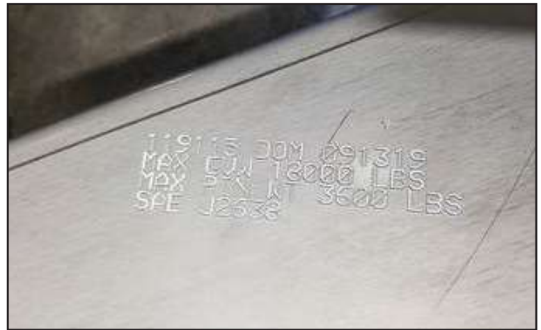
Fig.2 Dot Peen Before Powdercoating
