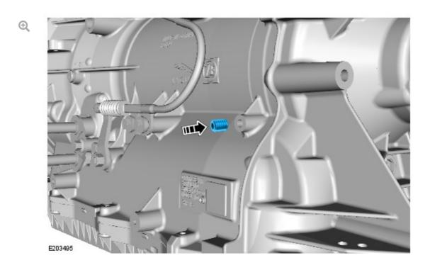
Apply Loctite 542 or equivalent to the new grub screw and install the new grub screw.
