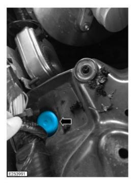
Install a body sealing plug (T4A8418/LR132021) into the hole on the right suspension top mount assembly, highlighted in the illustration.
