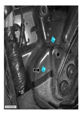
Remove the backing and install a sealing patch over each small hole.
