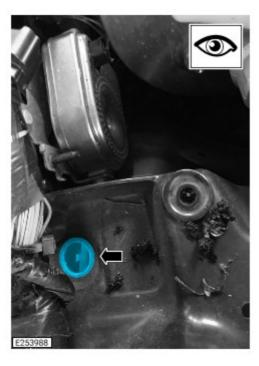
Locate the hole on the right suspension top mount assembly, highlighted in the illustration.
