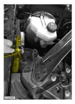
Reposition the engine compartment wiring harness on the right of the engine compartment.
