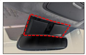
If the existing rain module and sensor assembly part number (A) does <u>not</u> match (P/N 96000 J3000), remove the existing rain module and sensor and replace it with the 96000 J3000FFF part listed in page 5 as outlined on KGIS.
