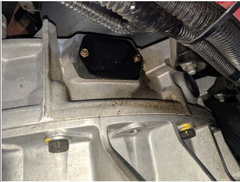
Figure #1: A26 Light Oil Film Present at Lower Flywheel Housing
