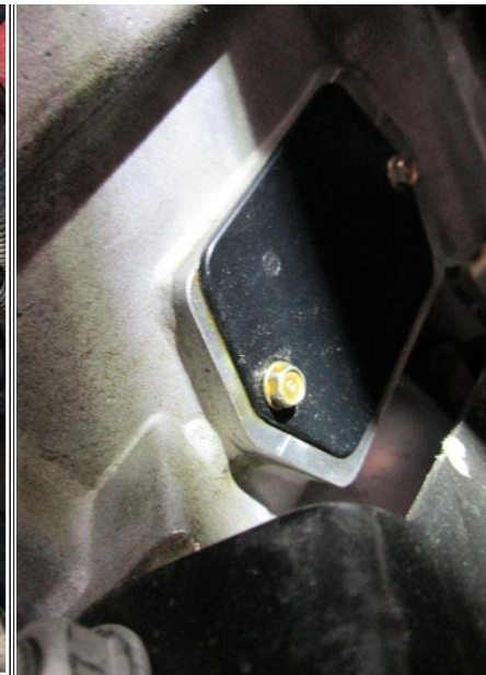
Figure #2: A26 Light Oil Present at Inspection Cover
