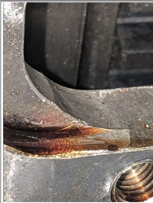
Figure #4: A26 Light Oil Collected under Inspection Cover
