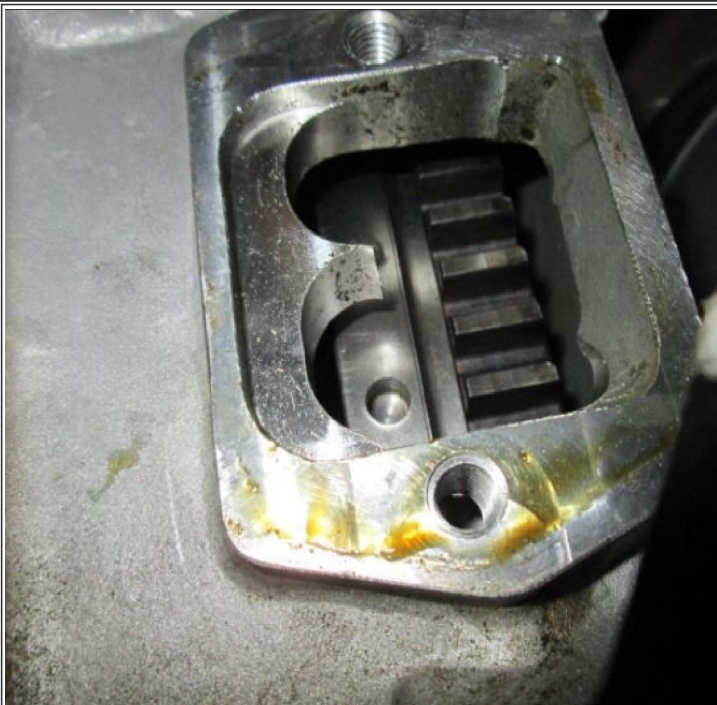
Figure #3: A26 Light Oil Seen with Inspection Cover Removed
