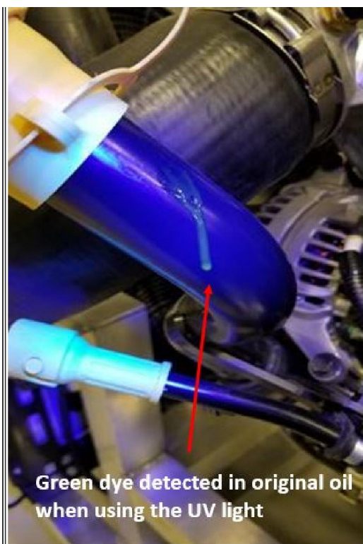
Figure #6: Example of dye's reaction to the UV light
