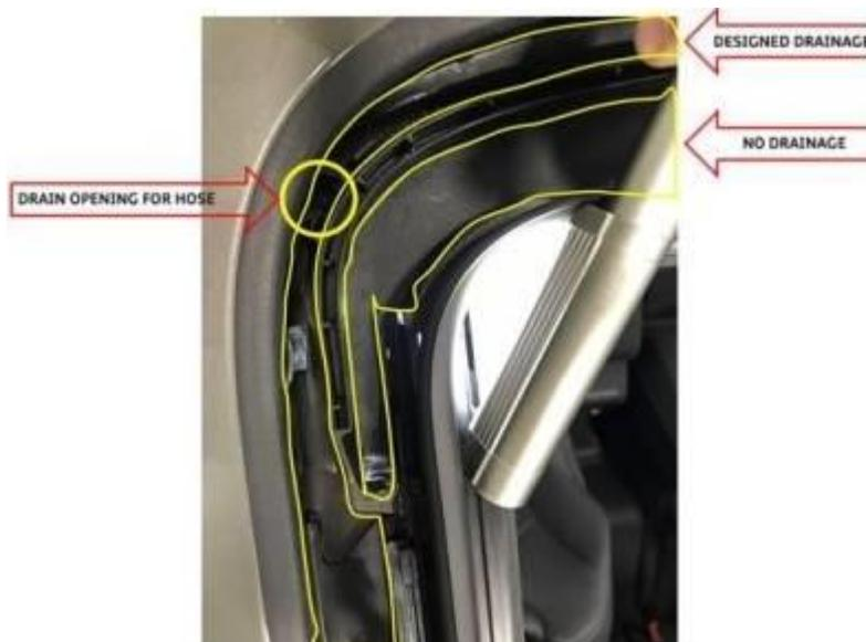
**Figure 4.** Sunroof water channeling diagram.
