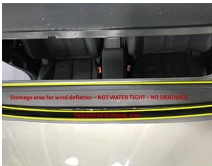
**Figure 3.** Areas of sunroof opening water elimination capabilities.
