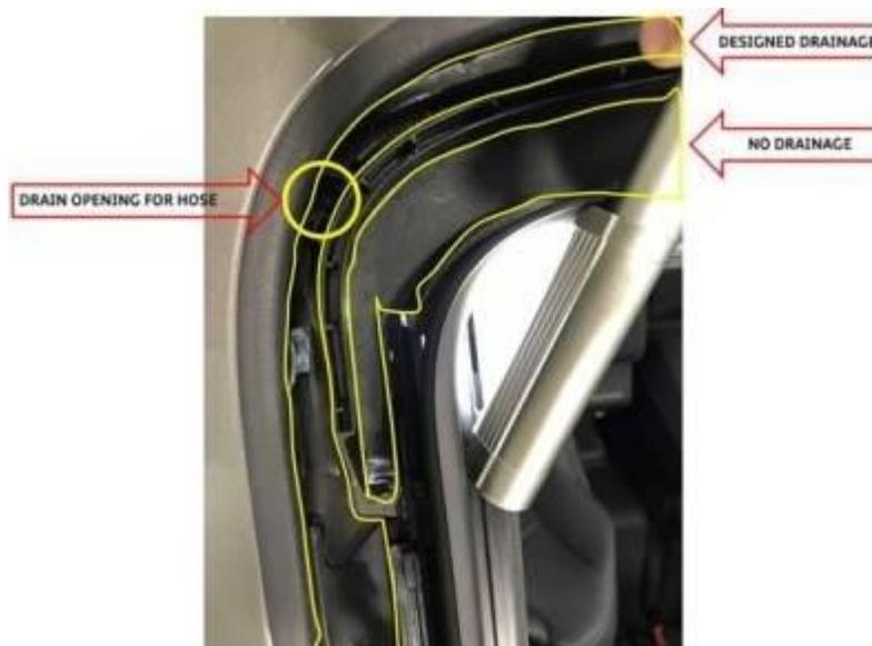
**Figure 4.** Sunroof water channeling diagram.
