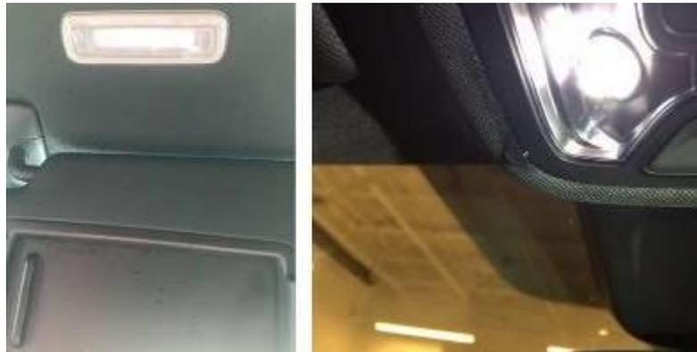
*Figure 1. Water intrusion near the headliner.*
