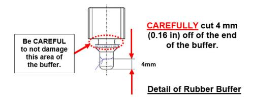
• If the buffer has a short projection as shown in Fig. 2 above, proceed to Step 4.
