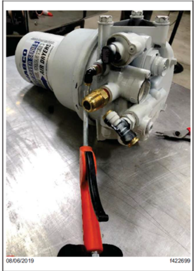
Fig. 5, Applying Shop Air to Dislodge the Valve
