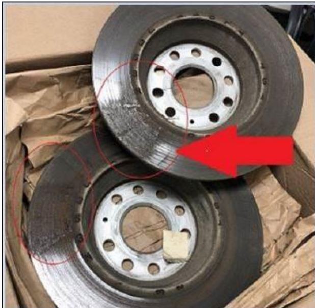
Figure 9: Brake Pad stuck to Brake Disc
