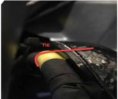
**If the wiring harness is found to be damaged:** Repair the harness using pigtail(s) part number 23662347 (chassis side) and/or part number 23662349 (hood side).
