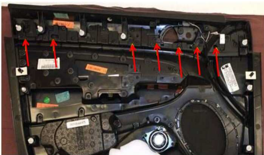
Fig. 11 Six Retaining Screws on the Rear Door Panel
