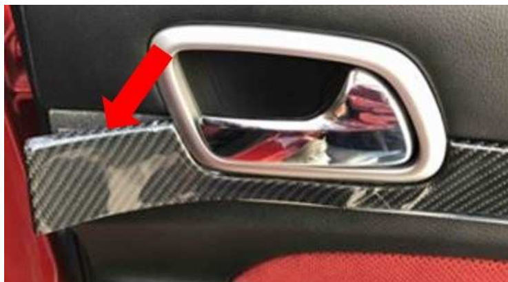
Fig. 1 Carbon Fiber Applique Delaminating Example
