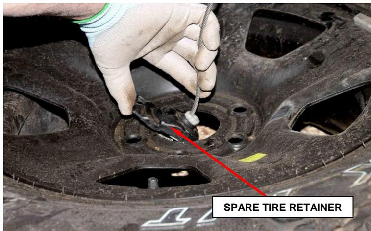
**Figure 9 – Spare Tire Winch Release**
