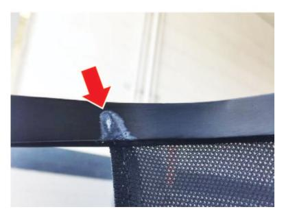
There's no need to replace the wind deflector. Just wipe away the residue with a damp, commercially available magic eraser or similar product, and dry the mesh fabric before closing the panoramic roof glass.
