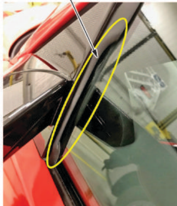
OUTER DOOR SEAL PINCHED
