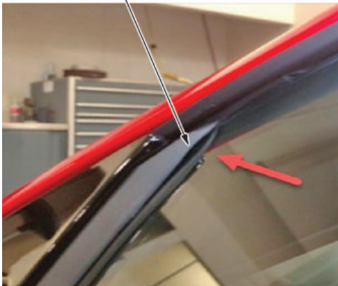
OUTER DOOR SEAL GAP
