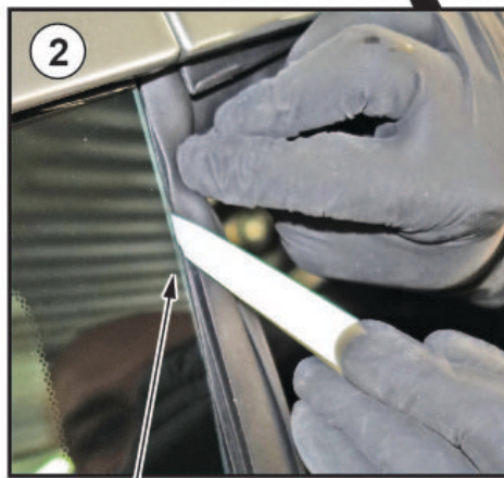
Ensure the door seal lip fits into the gap using a plastic stick.
