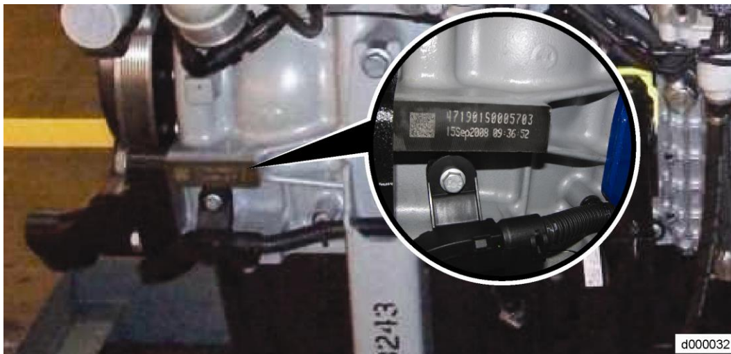
Figure 1- Engine Serial Number Location on Engine Block
