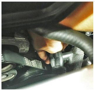
3. Locate the lower heater hose and check the distance between the drive belt and the heater return hose. A finger should fit between the drive belt and the heater return hose. If a finger fits, the clip of the heater return hose is correctly fastened.
