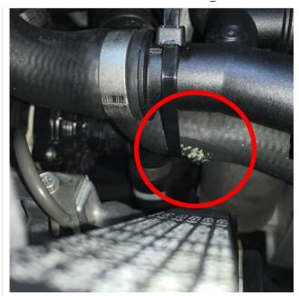
If it is already scoured or shows other evidence of abrasion (circled), it must be replaced
