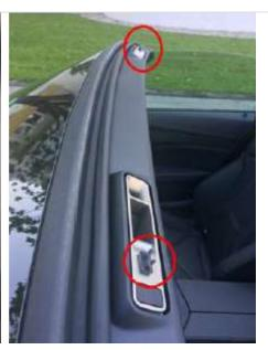
Rubber bumper pads (circled) are normally attached to the latch on the convertible top. Under certain circumstances, one or both pads stick to the corresponding latch plate above the windshield, pulling away from the latch. This can also cause a check control message 270 stating that the soft top is not locked.
