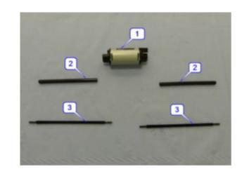
Remove the drive shafts from the seat track assembly.
