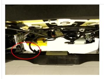
Disconnect seat motor electrical connector.
