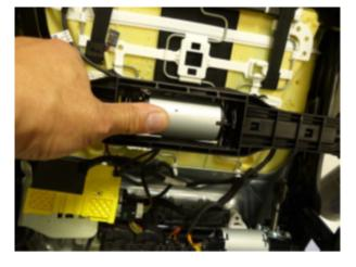
• First remove the electrical connector side from the plastic tray
