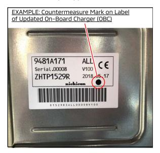
NOTE: The countermeasure OBC part (p/n 9481A171) should have a mark (black dot) on the label, as shown.
