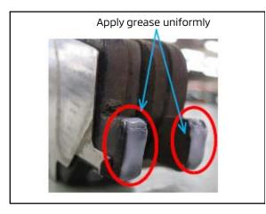
!! IMPORTANT !! Apply grease uniformly so that the base of the brake pads are completely covered with grease, as shown.
