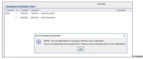
**Note:** If the Same Calibration/Software Warning is noted on the SPS Summary screen, record the warranty claim code (WCC) and select OK and follow screen instructions. After a successful programming event, the WCC is located in the Service Programming System dialogue box of the SPS Summary screen. No further action is required. Refer to the Warranty section of the bulletin.
