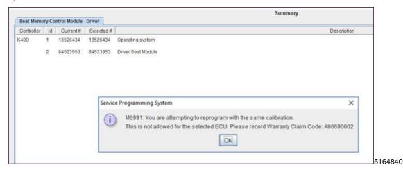
**Note:** If the Same Calibration/Software Warning is noted on the SPS Summary screen, record the warranty claim code (WCC) and select OK and follow screen instructions. After a successful programming event, the WCC is located in the Service Programming System dialogue box of the SPS Summary screen. No further action is required. Refer to the Warranty section of the bulletin.
