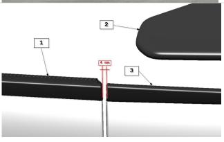
Firmly press the side trim onto the vehicle body, ensuring all 3 clips of the side trim are completely installed.
