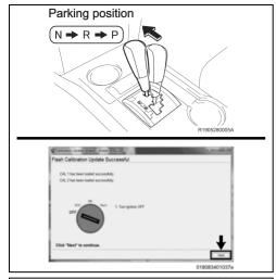
m) After "Flash Calibration Update Successful" is displayed, move the shift lever to Parking position and turn the IG off and click the "Next" button.
