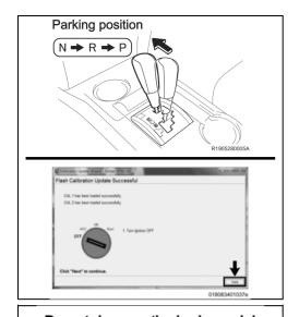
j) After "Flash Calibration Update Successful" is displayed, move the shift lever to Parking position and turn the IG off and click the "Next" button.
