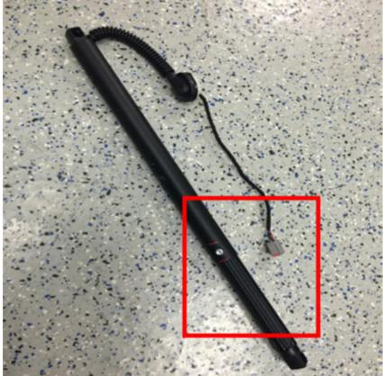
Note: The screw will hold the actuator together for removal.
