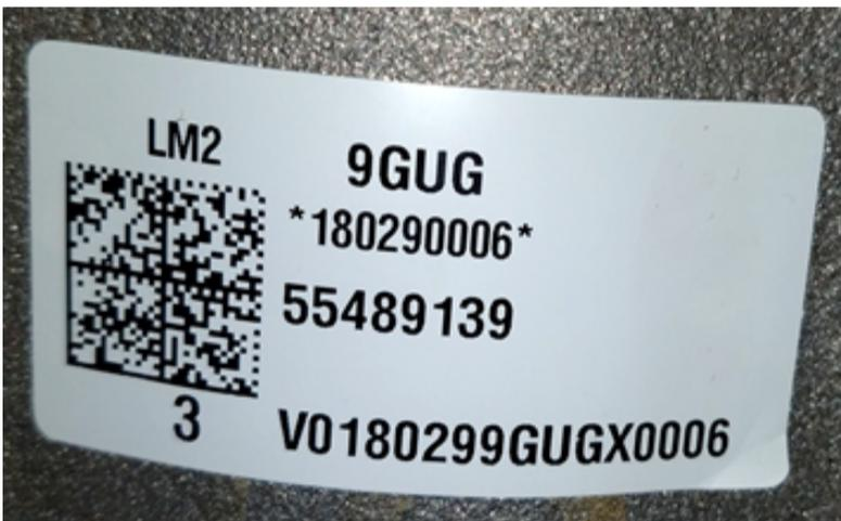
As shown in the above photos, the engine broadcast code can be found on the engine front.
