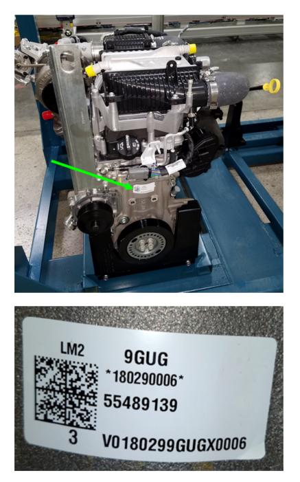
As shown in the above photos, the engine broadcastode can be found on the engine front.
