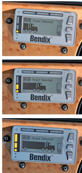
Figure 9 - Bendix™ Driver Interface Unit (DIU™) Showing Examples of Following Distance Alerts with Progressively Faster Audible Alerts
