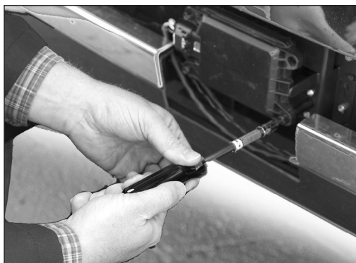
ABOVE: A TECHNICIAN MAKES AN ADJUSTMENT TO THE LATERAL ALIGNMENT STANDOFF.
