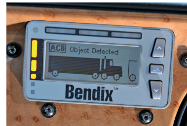
Figure 11 - Stationary Object Alert (SOA) Displayed
