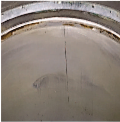
Examples of bore discoloration
