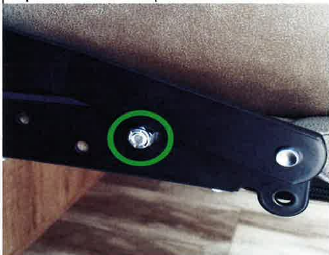
Stop Bolt Installed Example
