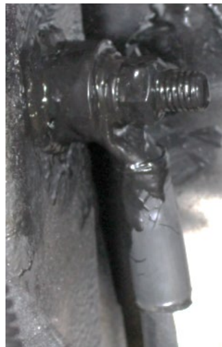
FIGURE 126: GROUND STUD WITH RUBBER COATING
