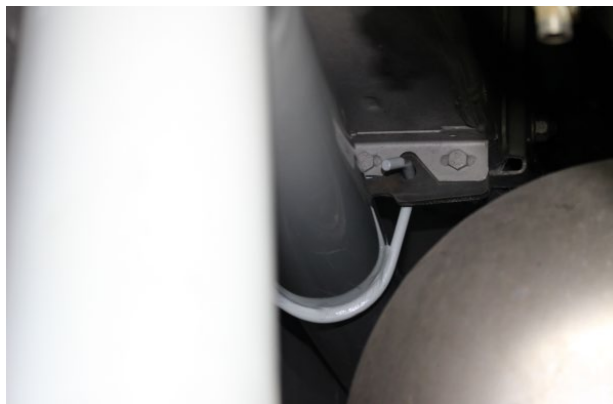
FIGURE 99: ENGINE INTAKE PIPE SUPPORT
