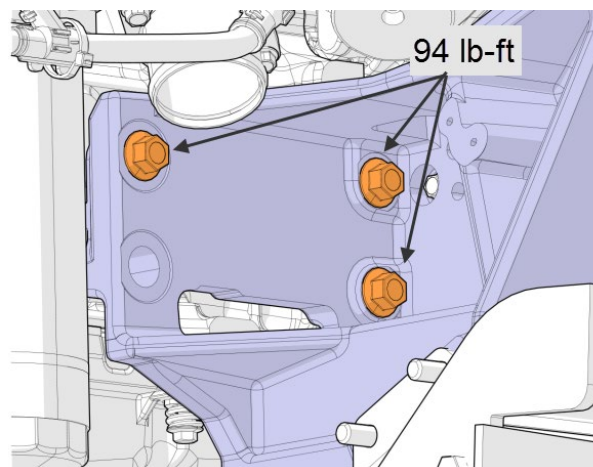
FIGURE 56: THREE (3) SCREWS ON THE SIDE OF THE ENGINE MOUNT
