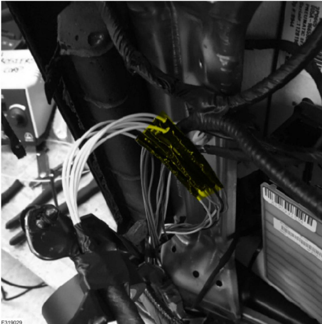
5. Wrap the new wiring with Coroplast tape or equivalent from the plastic harness shield to the connector.
