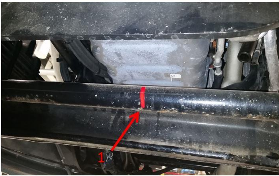
Figure 1: Tie rod assembly
