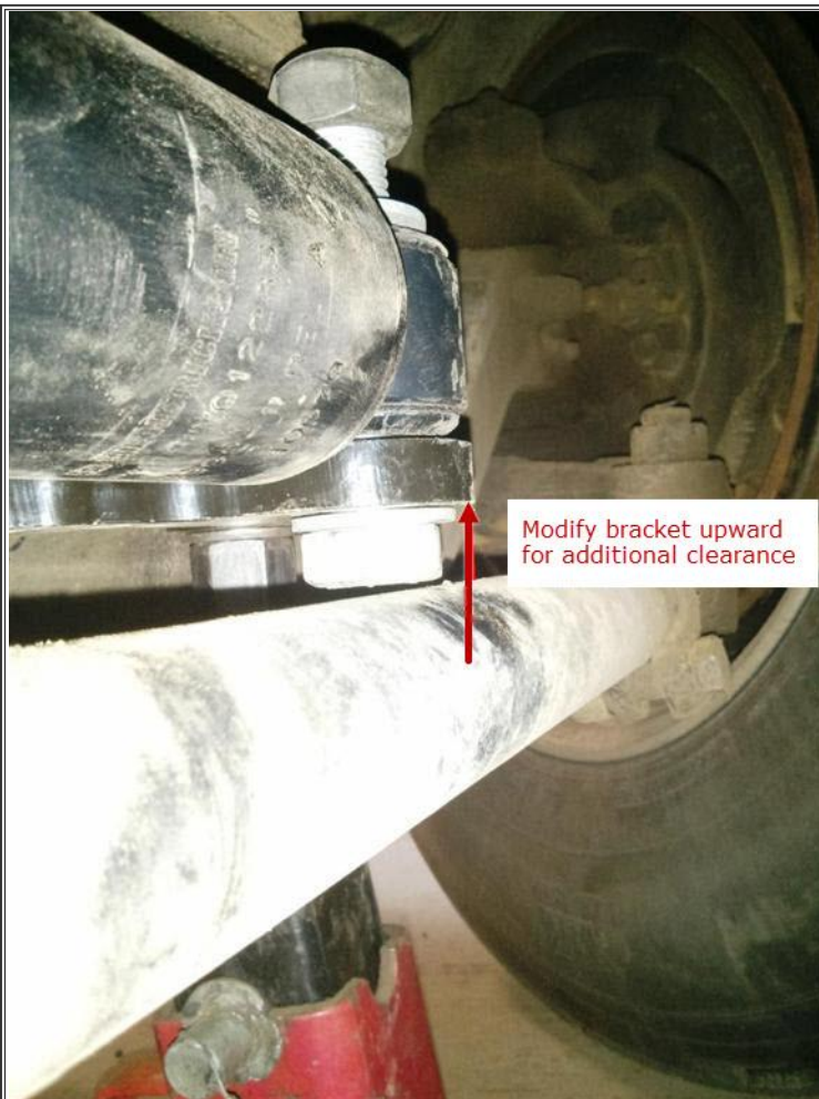
Figure 4: Tie rod tube to mount clearance
