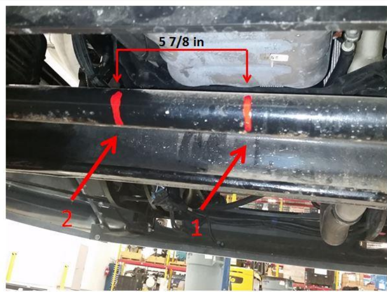
Figure 3: Tie rod assembly
