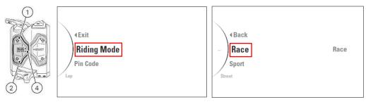
Any time you press **buttons (1)** or **(2)**, the instrument panel will display the riding modes and the "EXIT" indication. Once the desired "Race" Riding Mode is selected, press **button (4)** to confirm.
