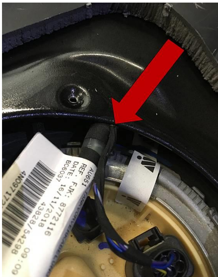
Figure 1. Location to inspect for rub through.
