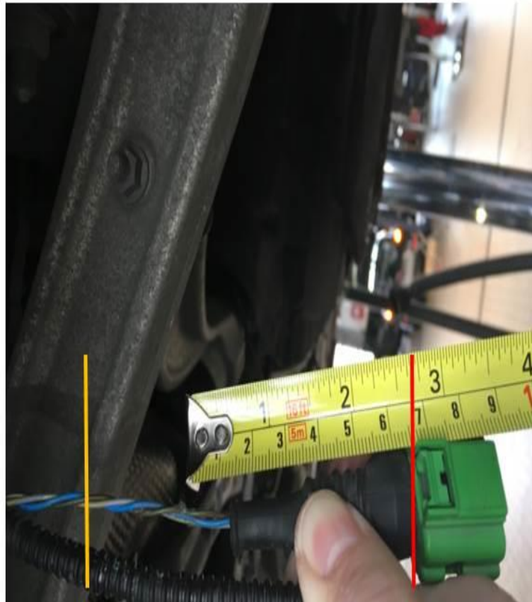
Figure 1. The affected area located under the corrugated tube between the red and yellow mark.
