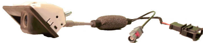
Figure 5. Completed reverse camera assembly with a new electrical harness.
